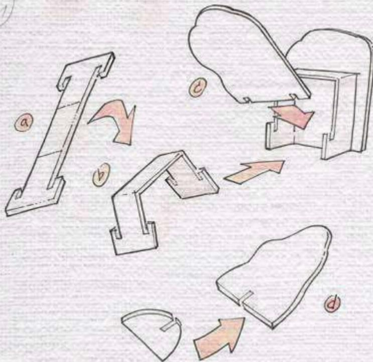
Each Ride is composed from **3 pieces**, marked by the same letter: a central structure with **bendy parts** and the two sides. Assemble them as depicted in the illustration to the left, there's no need of glue. Knowledge of the alphabet and basic hand-eye coordination are still required, though.
